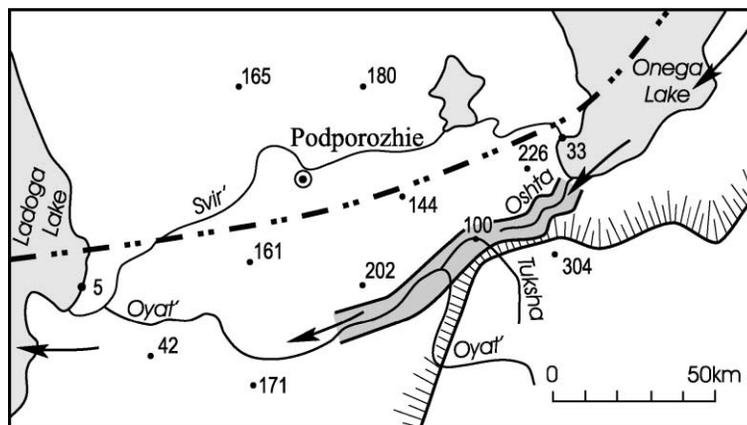
Fig. 6. The geomorphology on the Onega–Ladoga isthmus. For symbols, see Fig. 5. Buried valley mapped by Malakhovsky et al. (1995). Circle with dot indicates the location of the Podporozhie borehole where an Early Weichselian till is described (Zarrina et al., 1989). Arrows show possible spillway of the Lake Komi system towards the Baltic Sea.
