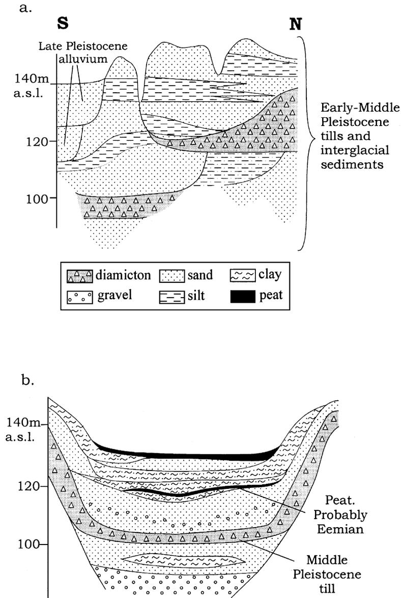
Fig. 3. Cross-sections of (a) the Mylva (simplified from Ryabkov, 1967) and (b) Keltma (simplified from Yakovlev, 1956) through valleys.
